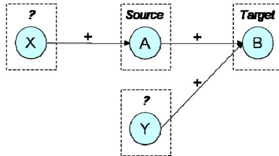
Figure 5.3: Hypothetical causal graph. Source quantity A has known behaviour, therefore quantity X should be left uninitialized not to cause contradictions. Quantity Y should however be initialized to zero or be removed to be able to calculate the effect of A on target quantity B.
