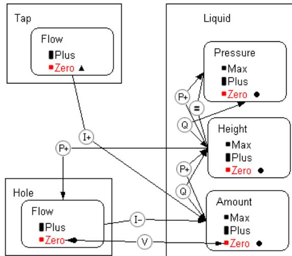
Figure 2.1: Dependency view of the contained liquid with in and outflow model. The tap has a flow that has a positive influence on the amount. Amount determines height and pressure. A hole in the container has a flow that negatively influences the amount in the container.
