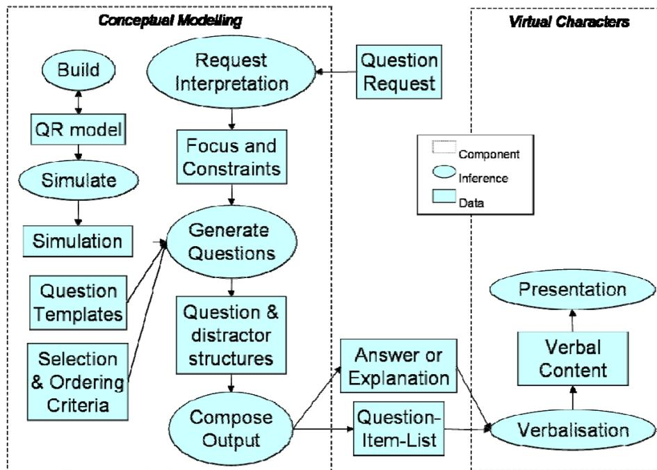
Figure 2.1: Context of the DynaLearn Question Generator component. The Question generator is invoked by a question request which is interpreted and which provides a focus for the main generator inference. Question structures are interpreted according to the request type to compose output that can be verbalised and presented.
