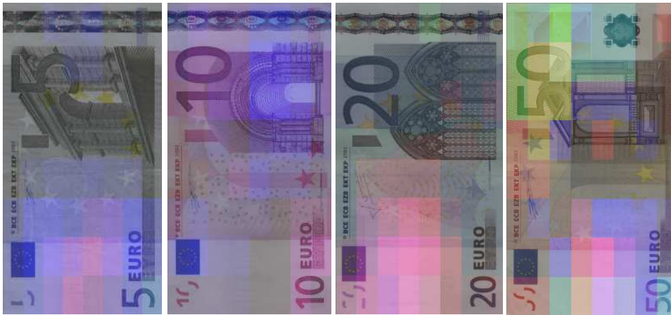
Figure 8 – Selected regions by BRAIN 2 on DeLaRue CPS 2000. The regions are overlaid over the respective colour channel to which the region corresponds. It seems that there is not one “fitness standard” for the 5, 10, 20 and 50 denominations. To discriminate well between fit and unfit for euro 5 and 10 BRAIN 2 uses to a large extend the blue channel, whereas for the euro 20 and 50 BRAIN 2 mainly uses a combination of all colour channels. Thereby BRAIN 2 retrieves most information out of the watermark area for euro 5 and 20. For euro 10 and 50 BRAIN 2 puts also emphasis on the printed area.
