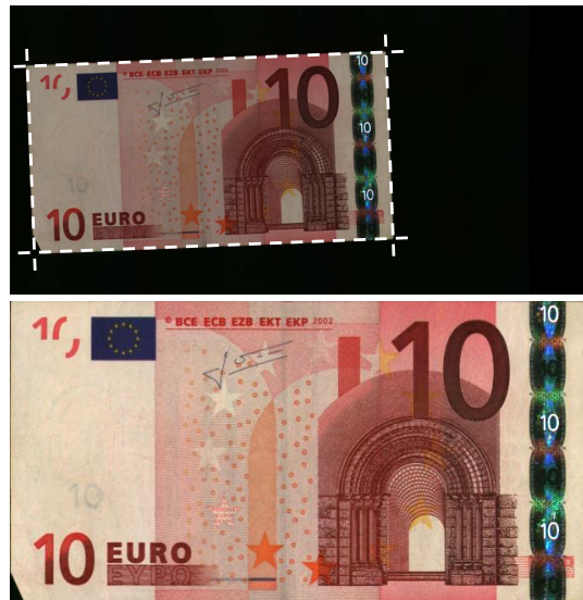
Fig. 2. The camera image with segment lines fitted through the contour (top) and the de-skewed banknote area (bottom).
