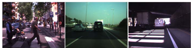
Figure 1. Vision-based road detection in real-world scenarios must be robust to extreme situations such as shadows, reflections, crowded scenarios or direct light source incident to the camera.
