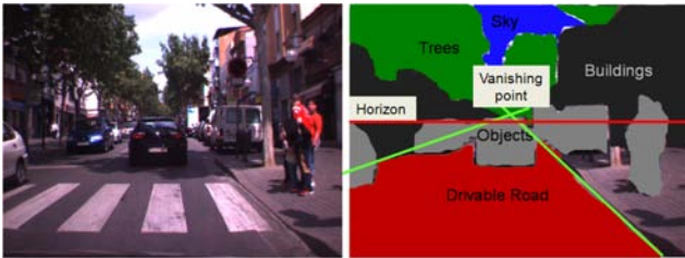
Figure 2. The proposed algorithm exploits all the information available in a single image to detect the drivable road surface ahead the target vehicle.
