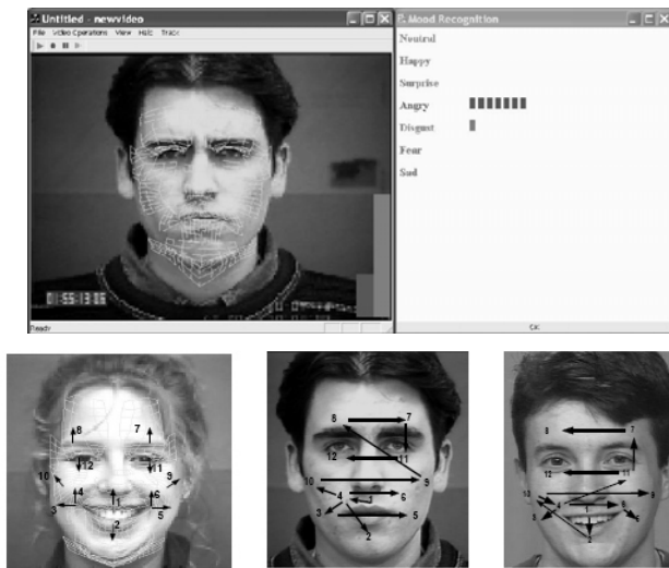
Figure 1. Our system’s interface (top) and the 12 motion units extracted. Each facial expression is assigned a probability value [0,1]. Arrows show correlations between motion units, learned when facial expressions are classified.
