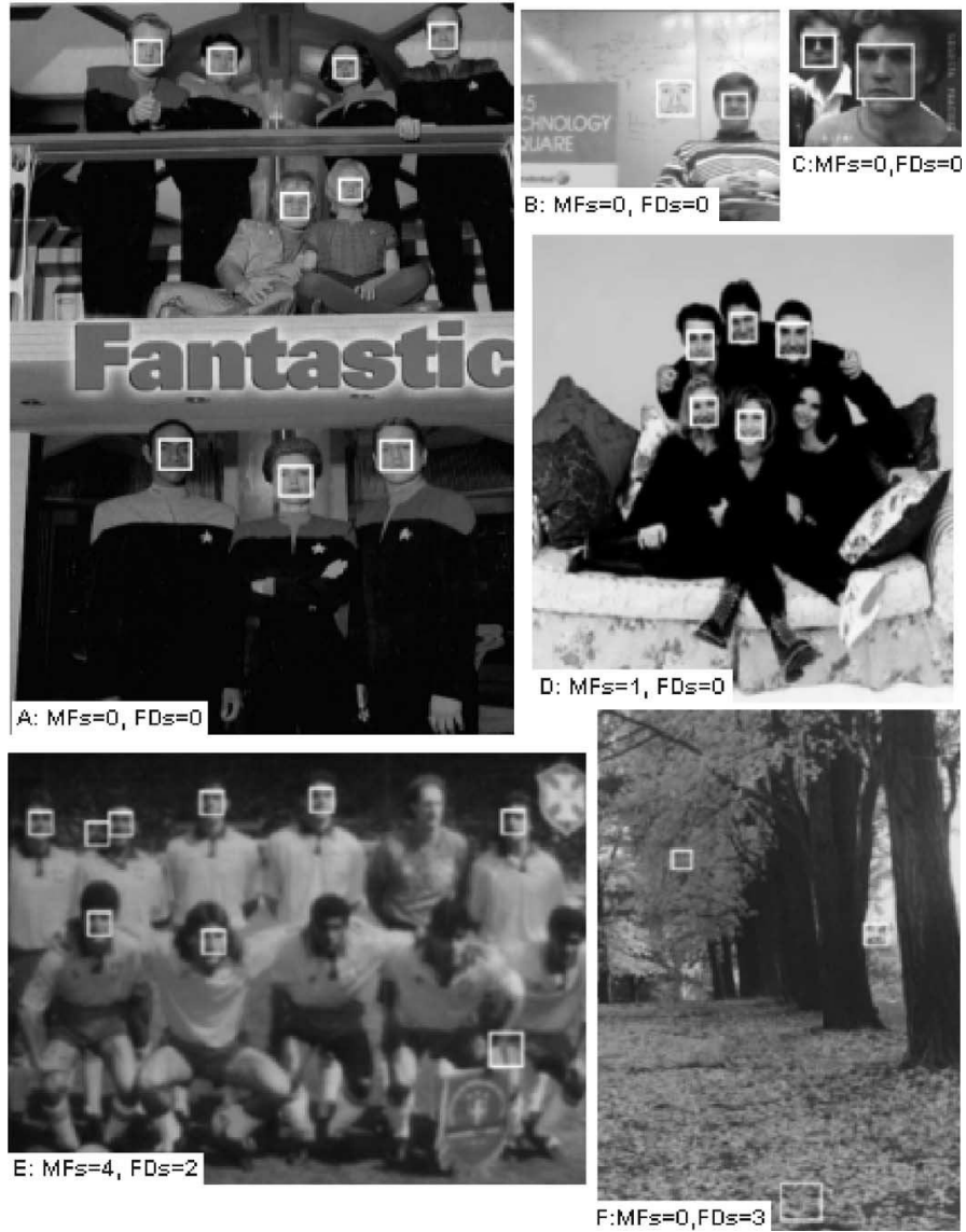
Fig. 3. Output of the system on some images of the CMU test using the SSS classifier learned with 19,000 labeled data. MFs represents the number of missed faces and FDs is the number of false detections.
