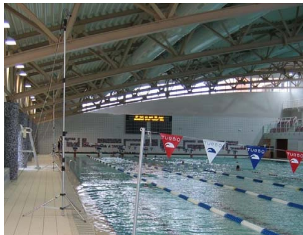
Figure 1. The hardware setup used to record the training session. The 3 PAL cameras are elevated at the pool side on tripods.
