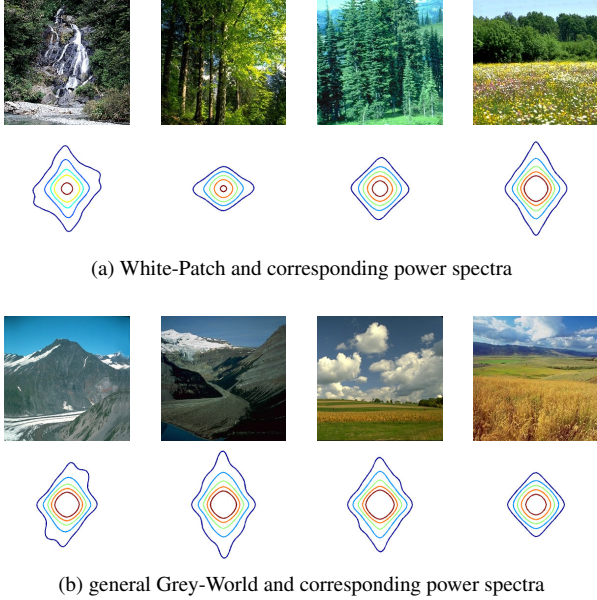
Figure 1. Examples of images on which the White-Patch algorithm (a) and the general Grey-World algorithm (b) perform better than other algorithms.
