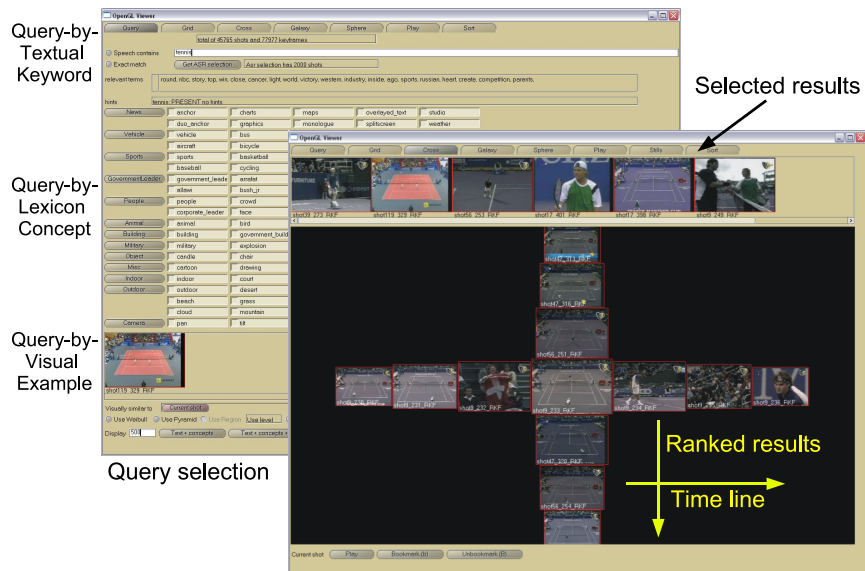
Fig. 3. Interface of the MediaMill semantic video search engine. The system allows for interactive query-by-concept using a large lexicon. In addition, it facilitates query-by-keyword, and query-by-example. Results are presented in a cross browser.
