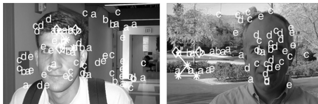
Fig. 8. Example of incorrect object localization. In both cases the part detectors fail to find a reasonable number of correct parts. In the image on the left only the left eye (denoted by letter b) is located correctly. In the image on the right, only the nose (denoted by letter c) is located correctly.
