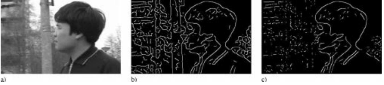
Fig. 3. (a) One frame. The object being tracked is the head of a man, (b) result of the Canny detector, and (c) removal of background edges according to (3).
